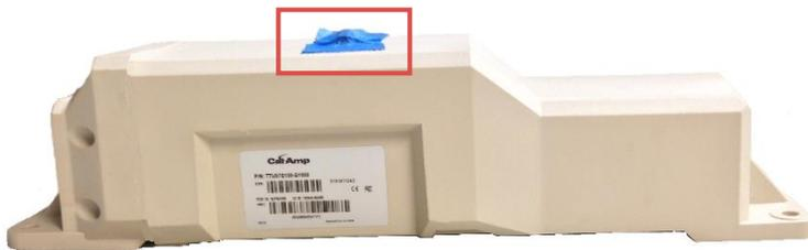
3. Remove the activation magnet. This should force the TTU-720 to wake and send a report.
